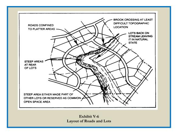
The master plan, or the transportation section of the master plan, provides the basis for classifying roads according to projected traffic flows. The same principle can be applied to subdivision and site plan roads, which must be designed to handle the projected traffic. All streets should be designed to meet construction standards prescribed by a local ordinance or the subdivision regulations.
